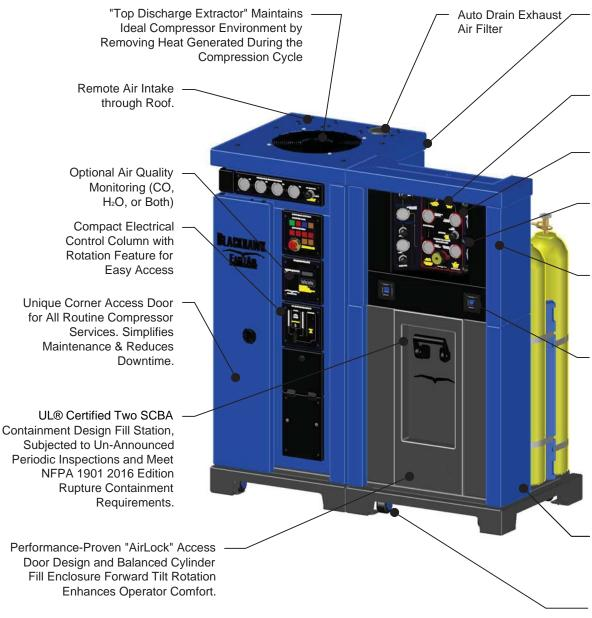
Integrated System is Designed for Against-the-Wall Installation and Accommodates up to Four (4) Air Storage Cylinders at the Rear of Unit.
